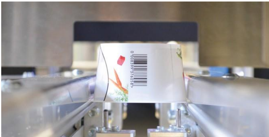
Making invisible defects visible: Non-destructive inspection of EVOH barrier layers
