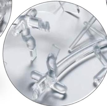
PMMA injection molding sprues
